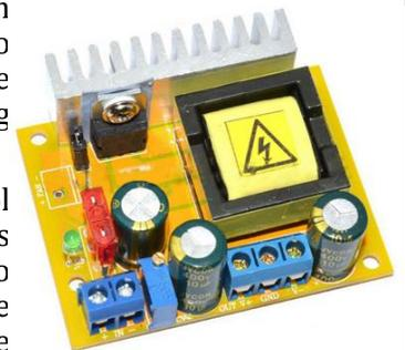
The PSU regulation is a little unstable with the very low leakage current and the high Capacitance, tending to inject some current then overshooting, turning off until the voltage dropped again. With a constant load current via a resistor it works much better, but no tests have been done to establish the limits of power and regulation or even how much noise is produced by the switching.
