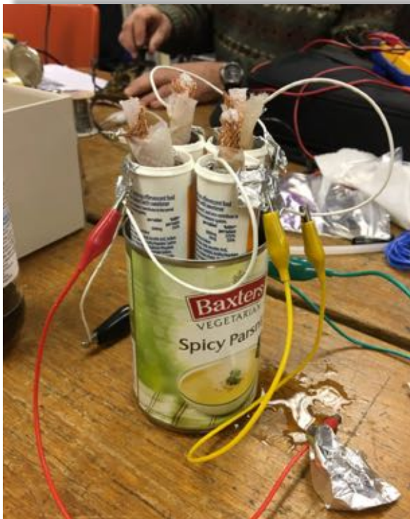
HARC's 'Spicy Parsnip' with a dash of vinegar plus salt battery which produced 2.35v
