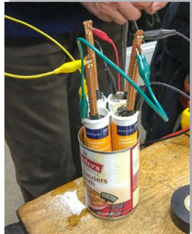
The CARC 'Highlanders Broth' battery also with a dash of vinegar & salt, which produced 2.8v
