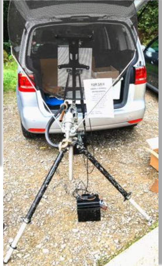
10GHz Antenna with 10GHz / 144MHz Transverter into an FT290
